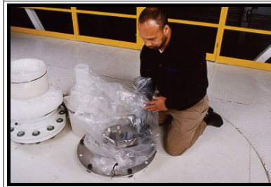
Attach the glove bag to the adapter Pad and the Dover Pac® system
