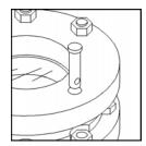
MANUAL LOCKING PIN: A locking pin goes through a small hole in the top plate of the Quickport<sup>TM</sup>. This blocks the path of the window ensuring the unit can not be opened while the pin is in place. This pin can then be locked with a standard  $\frac{1}{4}$ " padlock for extra safety.
