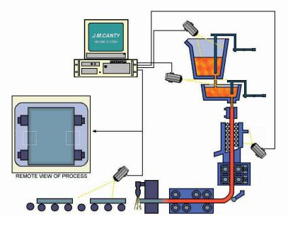
**CUSTOMER PROBLEMS:** Controlling the cutting process efficiently is critical in a continuous casting process. As the torch carriage rests on the slab it must index the edges mechanically in order to control the movement of the torches. Any error due to mechanical failure can cause incomplete cutting of the slab and a shut down of the line.
