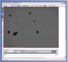
Step 3) The software then determines a threshold for the image, and each individual particle within the image is digitally mapped and analyzed. The major diameter, minor diameter, area and perimeter are measured, and logged into an EXCEL spreadsheet for each particle detected.
