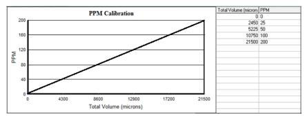
Therefore, when the total volume of particulate over a set number of frames is measured by the software, it can simultaneously output the associated ppm value. This visual calibration can be adjusted to match the operators lab technique if required.
