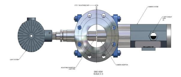
3. Probe Style System (24"+ Pipelines)
