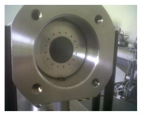
possible) due to the fact there is no danger of the glass and metal separating into 2 separate components. A jet spray ring is also included as standard in the system as a means of flushing the glass clean in the event that particulate does become lodged on the glass due to breaks in the flow etc.
