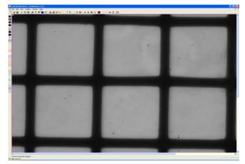
2 points on the grid displayed on the monitor are selected by the operator, and the known value of this distance is inputted to the software which then calculates the pixel scale factor. Therefore, any particle that shows up as 20 pixels wide for example, will be analysed by the software in it's real world micron value.
