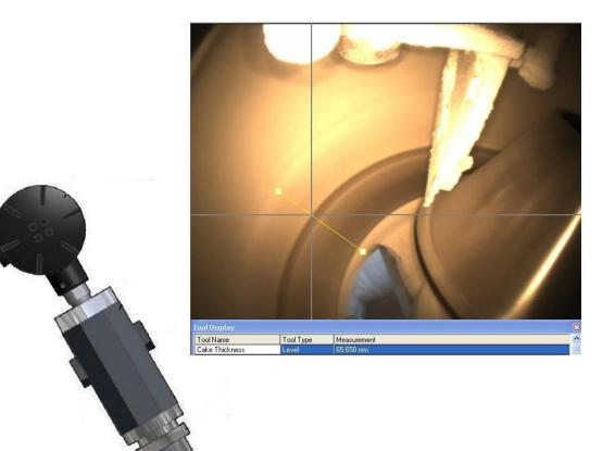
Ethernet camera & light combination unit provides remote view into the centrifuge for continual process monitoring
