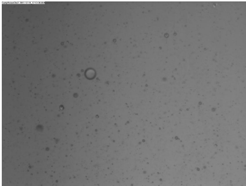
Figure 2 Live image of water droplets in oil (Approx. at 3,500 psi)
